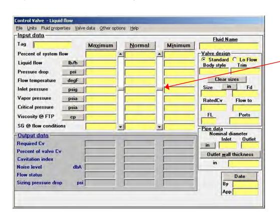
Based on changing percentage of flow, the program has a scrolling system to instantly give a variety of data calculations.
