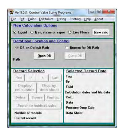
Contains programs for calculating Cv and analyzing for cavitation within the valve, critical flow and flashing through the valve, and noise generated by the valve.
