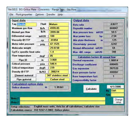
These programs determine the relationship between the flow rate, the pressure drop and the size of the hole.
