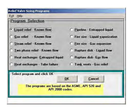
This liquid and gas application calculates API or ASME size for known flow, thermal expansion, and external fire.
