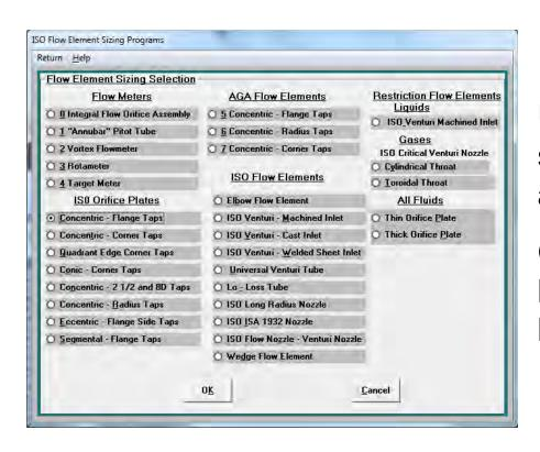
Uses concentric, eccentric, segmental, quadrant edge, and conical plates.
